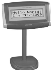
Figure 2.22 > Alphanumerical display 2x20 characters.
