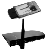
Figure 2.12 > Wireless communication: PCMCIA network card (top) and its access point (bottom).
