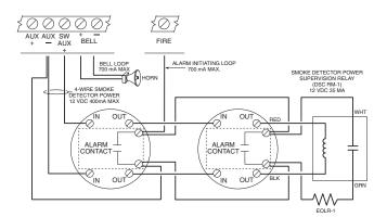
Smoke detector must be latching type (ESL 446C). To reset smoke detectors, press and hold [\*][4].
