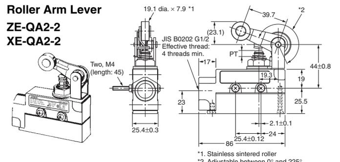
Note: 1. Unless otherwise specified, a tolerance of ±0.4 mm applies to all dimensions.
