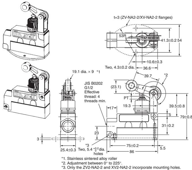
**One-way Action Sealed Roller Arm Lever**
