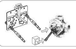
Example of mounting the actuator on mixing valve IKA.
