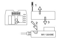
Relay module RM 24 is necessary to built in in case of controling the actuator with the room thermostat with one working (standstill) contact SPST. Functionally is RM 24 input relay for the actuator and output relay for the pump.
