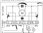
Power supply Rotation angle Rotation time for 90° Output torque Protection degree El. motor insulation class Ambient temperature Microswitch rating Connection cable lenght 230 V, 50 Hz, 3.5 W 90° 210s, 105s 6 Nm IP 55 120° 0 ... 55 °C 5(1)A, 250 VAC 5x0.75 mm², L=1500 mm
