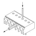
Loosen wire through twisting and pulling or using a Ø 1mm release tool
