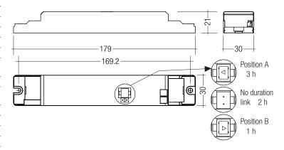
Note: LED Driver supplied with duration link in 3 hours position. Duration link must be set before battery and mains connection. The EM converterLED PRO 134 NiCd is supplied without a duration link.
