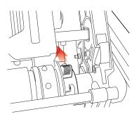
**3.** Adjust the right tractor to the paper width by pulling its lock lever forward, sliding the tractor to the desired position, then pushing the lock lever backward to lock it in place.
