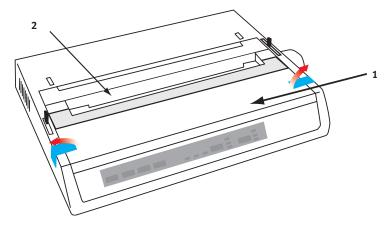
2. Remove the **printhead shipping restraint**. Keep shipping restraint for future use.
