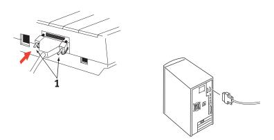
The cable should comply with the RS232C Serial Interface Specification and have a maximum length of 15 metres (49ft).
