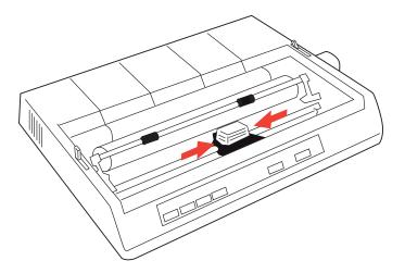
2. When replacing a Ribbon Cartridge, first remove the old one.
