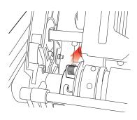
2. Adjust the left tractor if necessary, making sure that it is not more than 12.7mm (0.5 inch) from the left-hand end of the tractor unit. To move the tractor, pull the lock lever forward, slide the tractor to the desired position, then push the lock lever backward to lock it in place.
