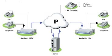
Calls Involving an Access Device and a LAN Endpoint The following examples illustrate how a phone/fax connected to a Mediatrix 1104 access device can communicate with a LAN Endpoint on the IP network.
