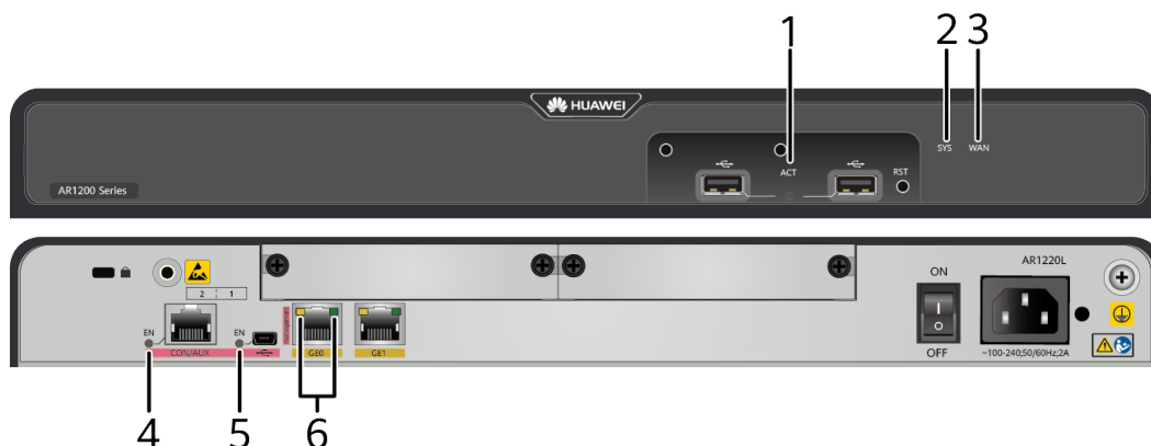
Figure 4-171 Indicators on the AR1220L
